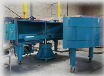
Laboratory Centrifuge with automatic centrifuge balancing mechanism
