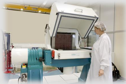
Two-axis Table. with climatic chamber and optical path for alignment
