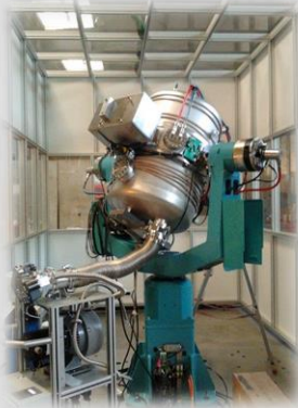
Two-axis with Combined Vacuum and Thermal Chamber for Space Technology
