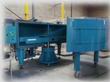
Laboratory Centrifuge with automatic centrifuge balancing mechanism
