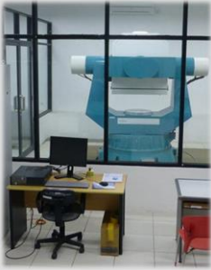
Three-axis Motion Simulator with climatic chamber
