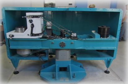
Laboratory Centrifuge with on board counter-rotating satellite rate table and temperature chamber
