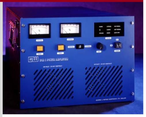
The DSA1 is a switched mode power amplifier based on the extremely reliable DSA4 design. The DSA1 is available in two output versions—1kVA or 2kVA. The amplifier is a compact size for bench top or rack mounting operations and incorporates the field supply and the degaussing supply for an electro-dynamic shaker. The amplifier is air cooled and may be remotely controlled for combined operations with a climatic chamber.
